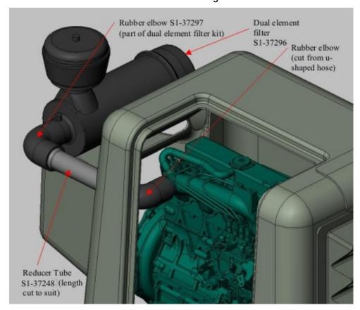
**Dual Filter Mounted Directly on Engine:**
