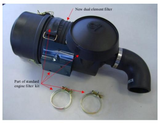
For Filter Mounted on Outside of Chassis:
